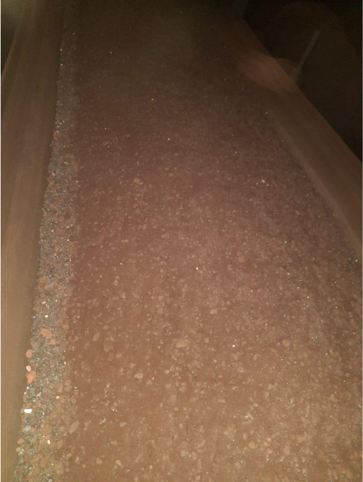
(BC-23 conveyor with oversize material)
