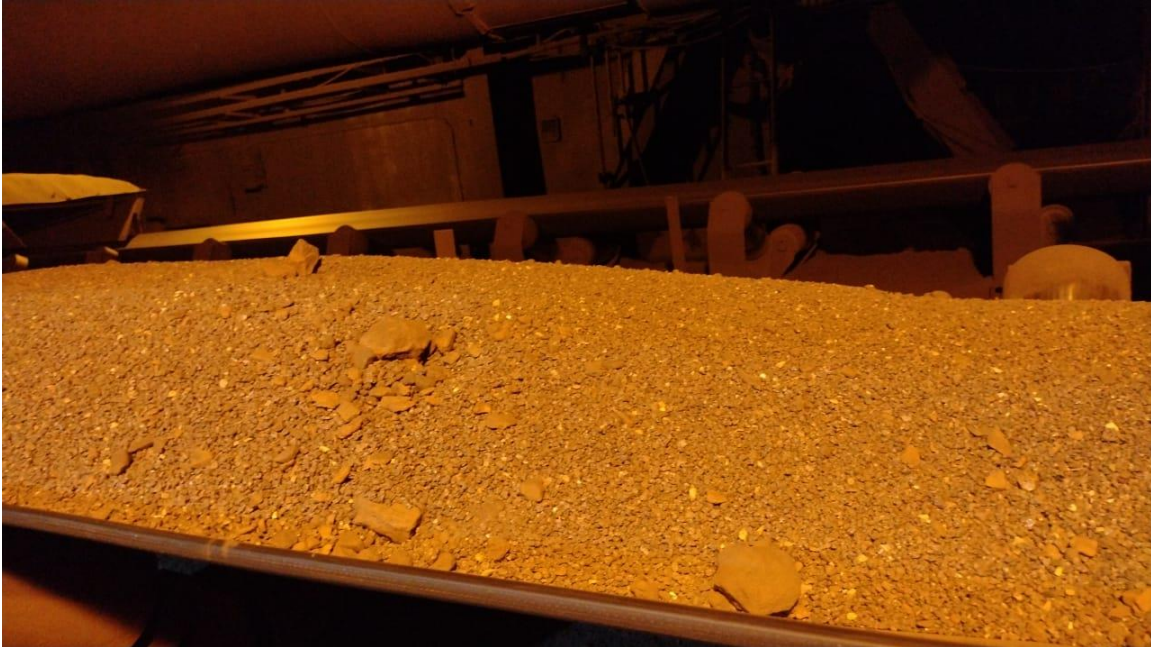
(BC-22 conveyor with oversize material)
